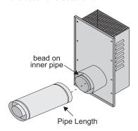
**10)** Seal around the outer edge of the Riser Vent Backing Plate.
